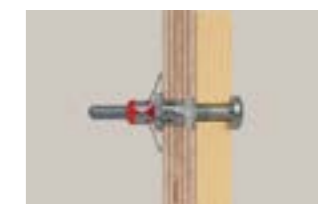
One plug length covers all common building material thicknesses from 9.5 - 30 mm, for flexible and cost-efficient application.
