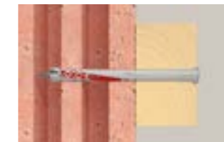
Application in perforated material
