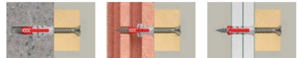
Intelligent self-activating functions depending on the base material.
